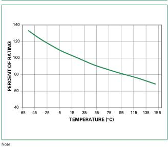
1. Rerating depicted in this curve is in addition to the standard rerating of 20% for continuous operation.
